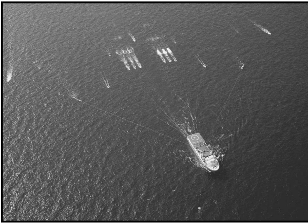
FIGURE 48. Seismic boat and streamers (courtesy of Woodside Petroleum, Web site: www.woodside.com.au .)
