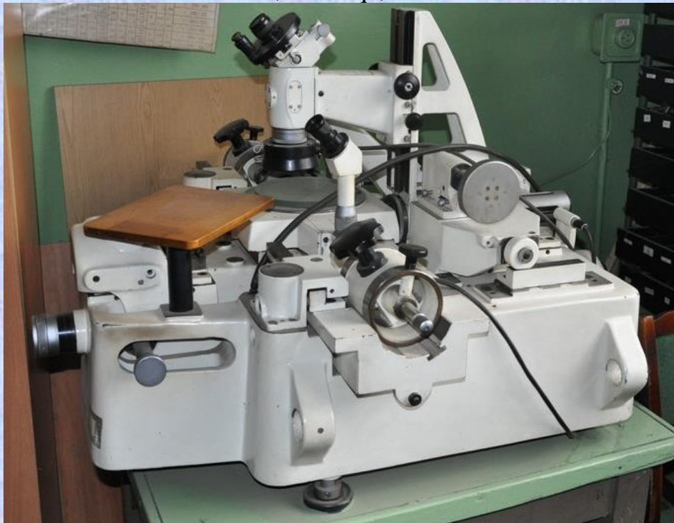
5.2-rasm. 5.1-rasm. UIM-21 universal o'lchov mikroskopining tuzilishi. 1-asos, 2-mikrovint, 3-karetk, 4-shisha shkala, 5-mikroskop, 6- sipiralsimon noniusli mikroskop, 7-vertikal kalonna, 8- mikroskop, 9-tubos, 10-maxovik, 11-karetk, 12-mikrovint, 13-maxkamlash vinti, 14-markazlovchi babka, 15-xalqa, 16-maxkamlash vinti.
