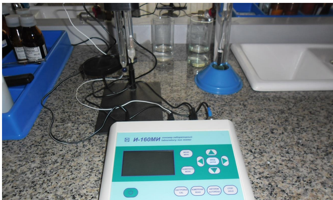
2.2.2-rasm. Maxsulot namunasidagi PX muxitini aniqlash uchun foydalaniladigan PX-MY va TDL-100 termodatchik.
