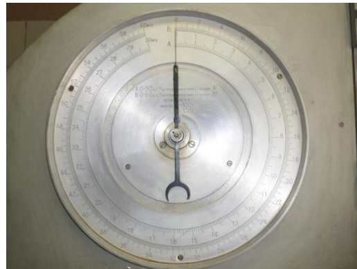
Rasm-1.4.5. RTI – 60 uskunasining kuchlanish darajasini o'lchagich .
