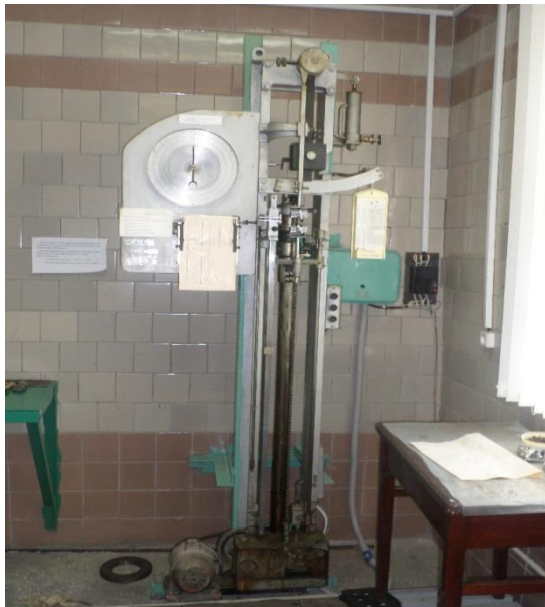
Rasm-1.4.5. RTI – 60 uskunasining kuchlanish darajasini o'lchagich .
