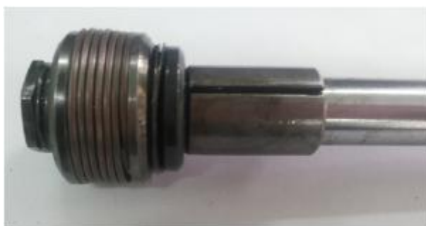
3.5-rasm. Piston birikmalari mis bilan qoplangan kamon
