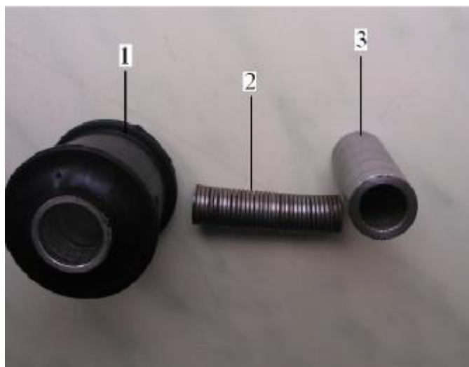
4.18-rasm. Innovatsion jim bloklar uchun ta'mirlash kiti qismlari 1 - jim bloklar, 2 konusning kamoni plyonkali, 3 - po'latdan buta Eksensional yuk qo'llanganda konusning kamoni diametri o'zgarishining natijalari (4.19-rasm).
