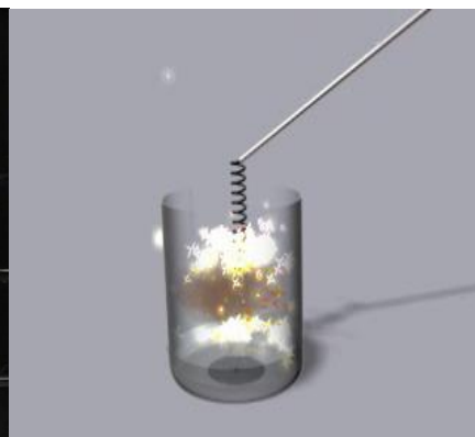
31-rasm. Ammiakning katalizator ishtirokida yonishi
