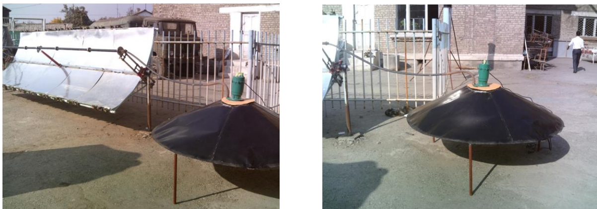
Fig. 3.2.6. Combined system collaboration parabolic cylindrical manifold with conical cylinder
