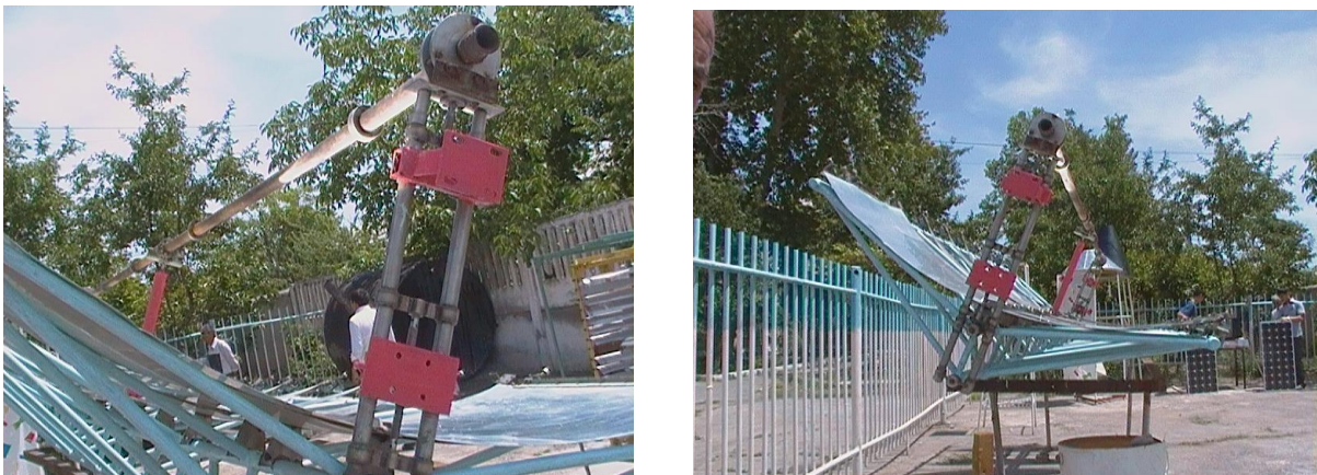
Fig.3.2.2. A heat energy module installation parabolic cylindrical
