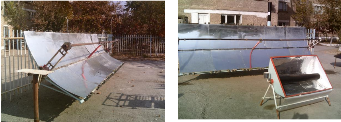
Fig. 3.2.3. Parabolic cylindrical energy module installation.
