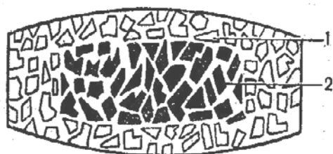
Rasm 4. Lontab turdagi tabletkalar tuzilishi
