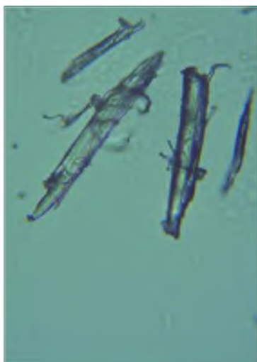
23- rasm. 3% HCl eritmasida termik usulda olingan GF zarrachalari tasviri(x400)
