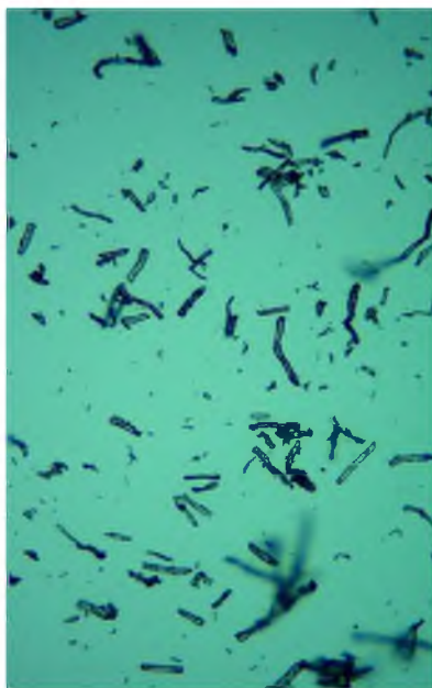
21-rasm. 3% KOH eritmasida termik usulda olingan GF zarrachalari tasviri(x100)
