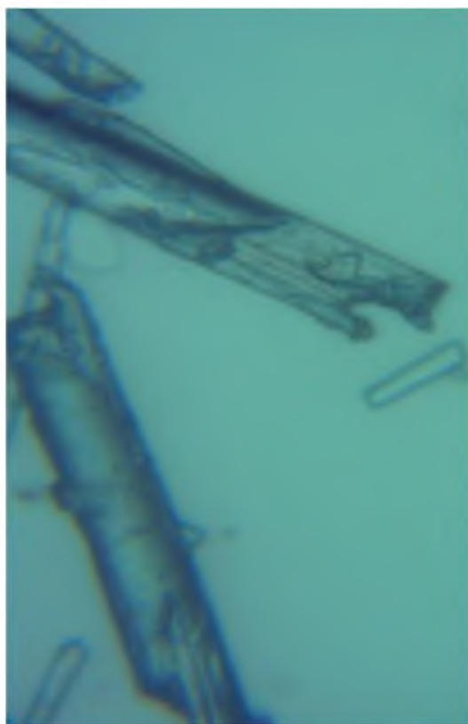
27- rasm. 3% HCl eritmasida 510 Vt quvvatli O'YCh nurlar ta'sirida olingan GF zarrachalari tasviri (x1000)
