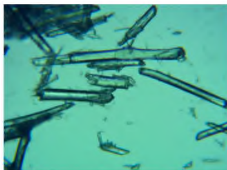
30- rasm. 3% HCl eritmasida 810 Vt quvvatli O'YCh nurlar ta'sirida olingan GF zarrachalari tasviri (x400)
