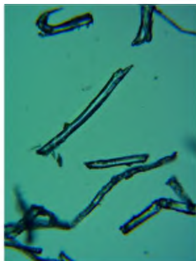
25-rasm. 3% NaOH eritmasida termik usulda olingan GF zarrachalari tasviri(x400)
