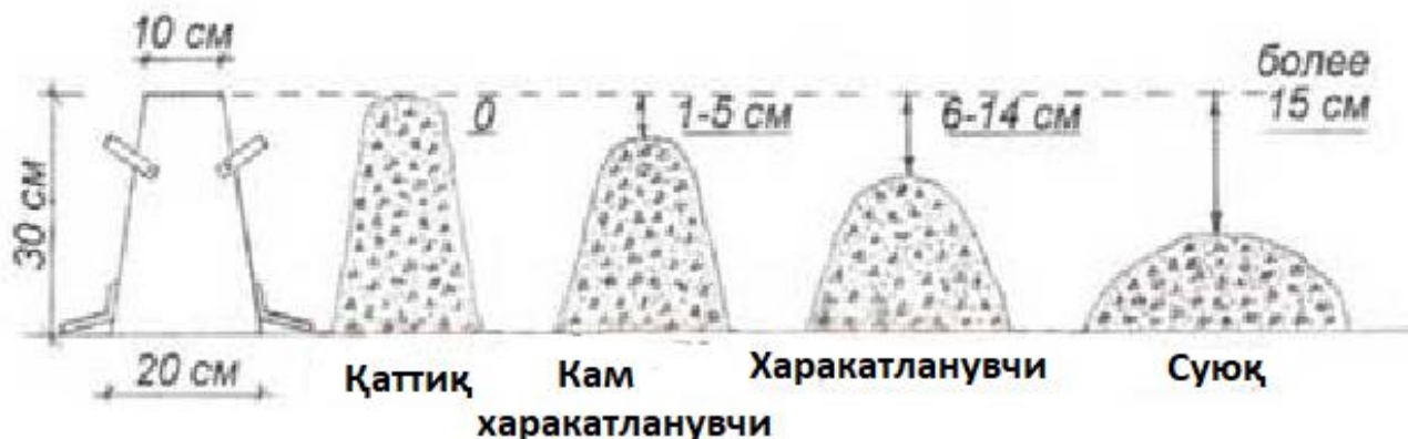
1-rasm. Beton aralashmaning harakatlanishini (konusning yog'lanishi) aniqlash sxemasi
