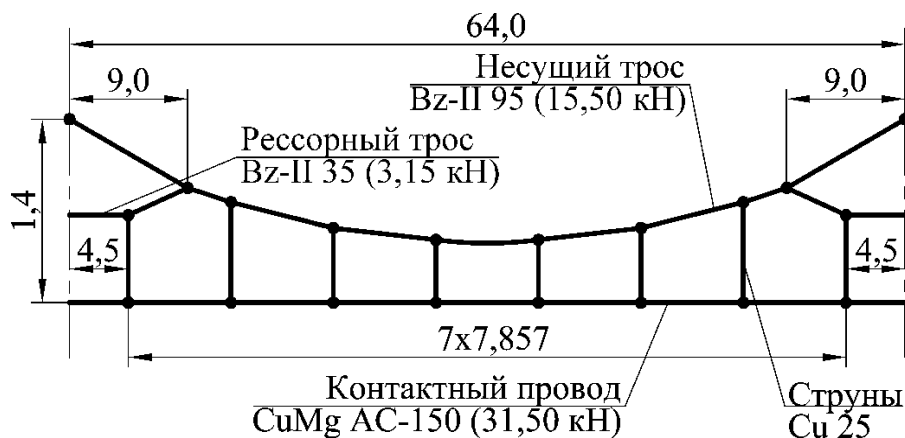
11.5-rasm. EAC-350 Ispaniyaning YuTM laridagi EAC-350 kontakt osmasining prolyoti sxemasi
