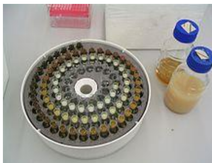
Fig.4. A rotary fraction collector collecting HPLC output. The system is being used to isolate a fraction containing Complex I from E. coli plasma membranes.
