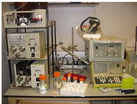
Fig.1. An HPLC. From left to right: A pumping device generating a gradient of two different solvents- a steel-enforced column and a detector for measuring the absorbance.
