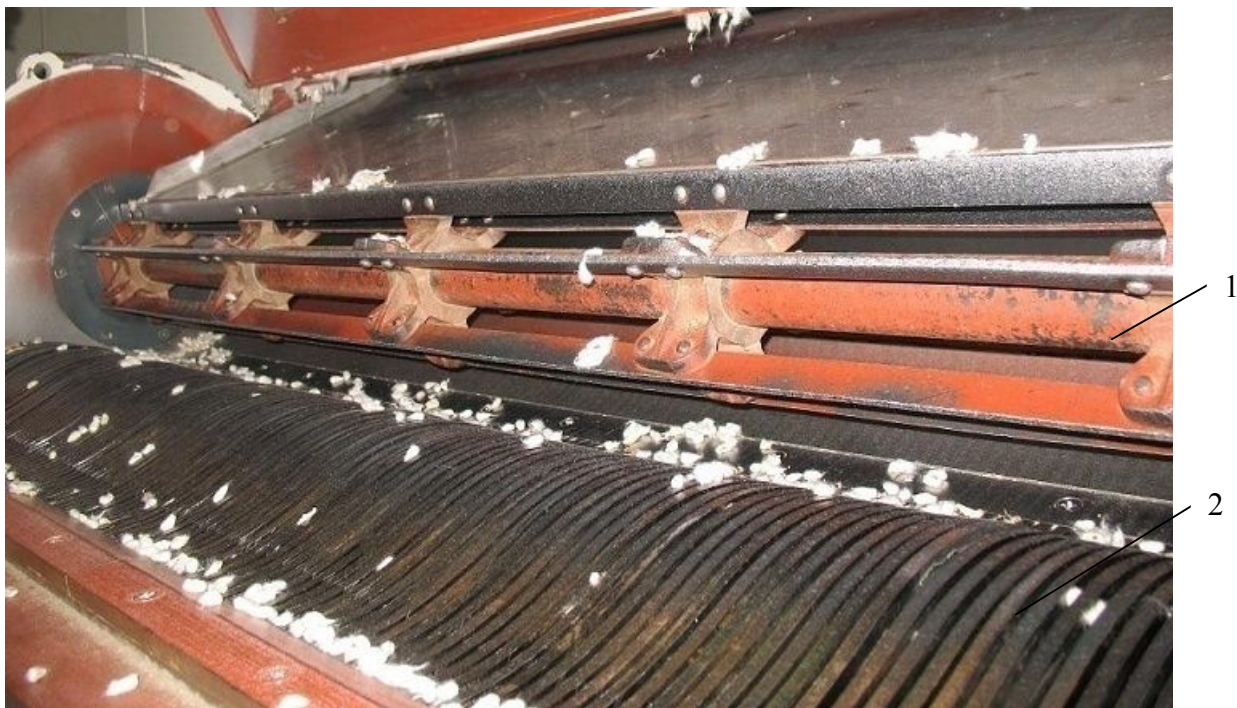
8-rasm. MR144D linterining ishchi kamerasi 1- to‘zitqich; 3- kolosnik panjara
