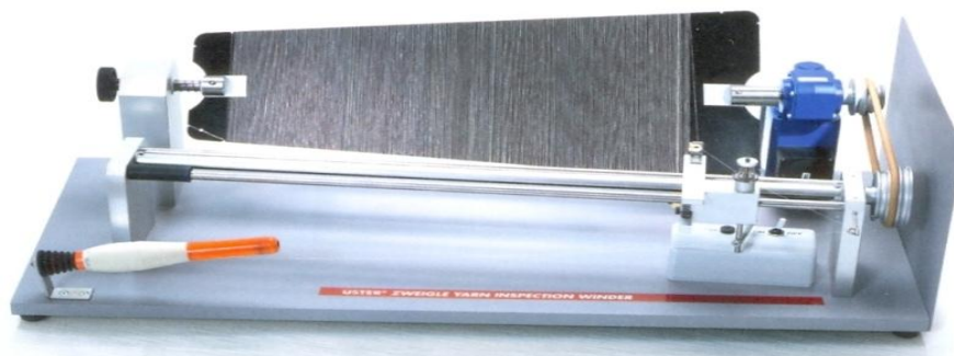
2.5-rasm. USTER ZWEIGLE YARN INSPECTION WINDER- Motovilo organoleptik usulda ipni sifati aniqlanadi
