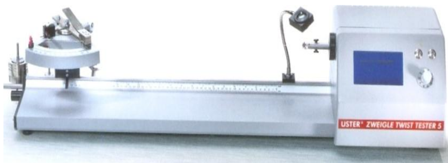
2.4-rasm. USTER ZWEIGLE TWIST TESTER 5- Ipdagi buramlar sonini aniqlaydi
