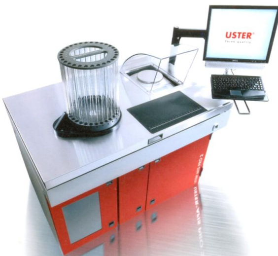
2.1-rasm. “USTER” firmasining AFIS PRO 2 sinov laboratoriya jihozi
