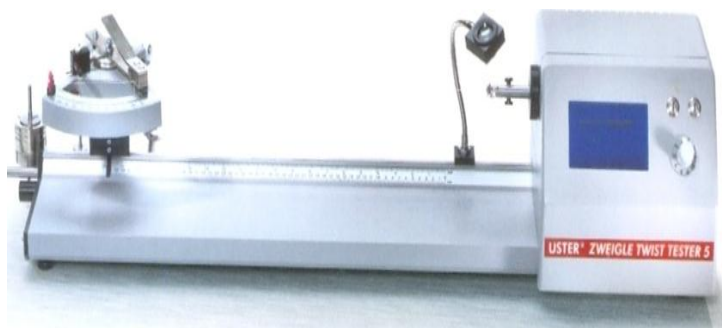
2.4-rasm. USTER ZWEIGLE TWIST TESTER 5- Ipdagi buramlar sonini aniqlaydi
