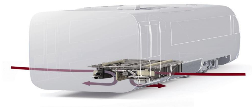
32.1.rasm. General Electric kompaniyasi lokomotivini sovutish sxemasi
