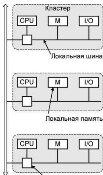
2.15-rasm. Cm* kompyuter tizimining sxemasi
