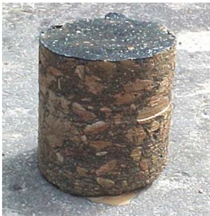
Figure 1.2. Pavement core proves strength of CTB
