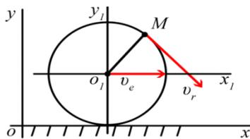
$v_A = v_B + v_{AB}; \quad v_{AB} = \omega r \ (r = AB)$
