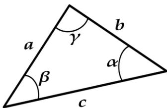
$$\frac{F}{\sin 75^\circ} = \frac{R_1}{\sin 60^\circ} = \frac{R_2}{\sin 45^\circ}$$
