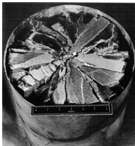
4-rasm. Litiy gidridning kristallanish jarayonida darz ketgan shakli
