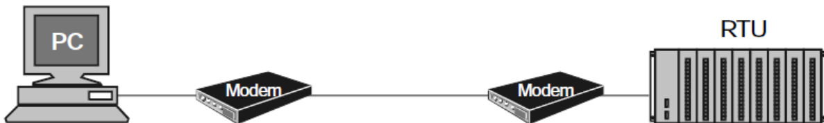
1.7-rasm. Kompyuterdan RTU ga modemdan foydalanish.
