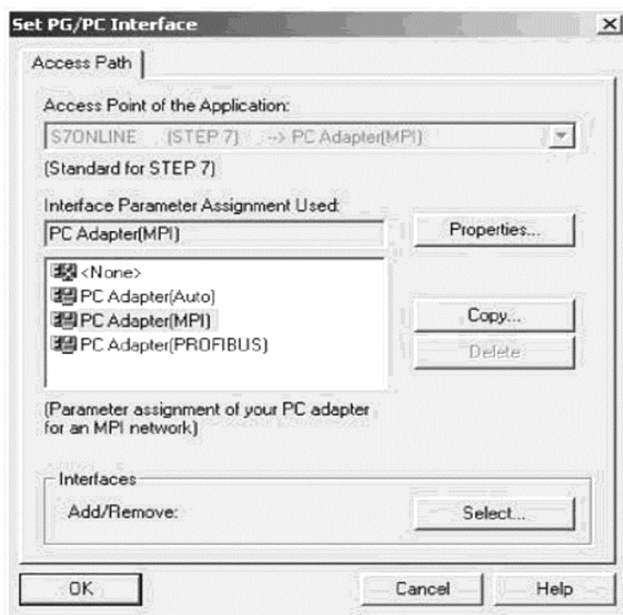
Rasm 1-19. PG/PC interfeys bog'lanishni aniqlovchi oyna.
