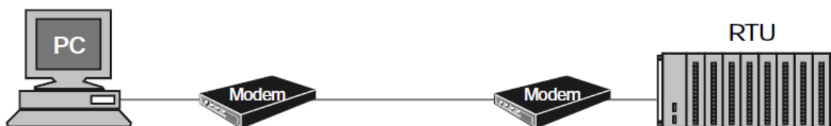
1.7-rasm. Kompyuterdan RTU ga modemdan foydalanish.
