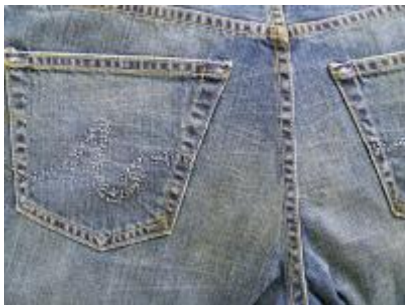
1.4.4 - rasm. Enzimlar bilan yuvish.
