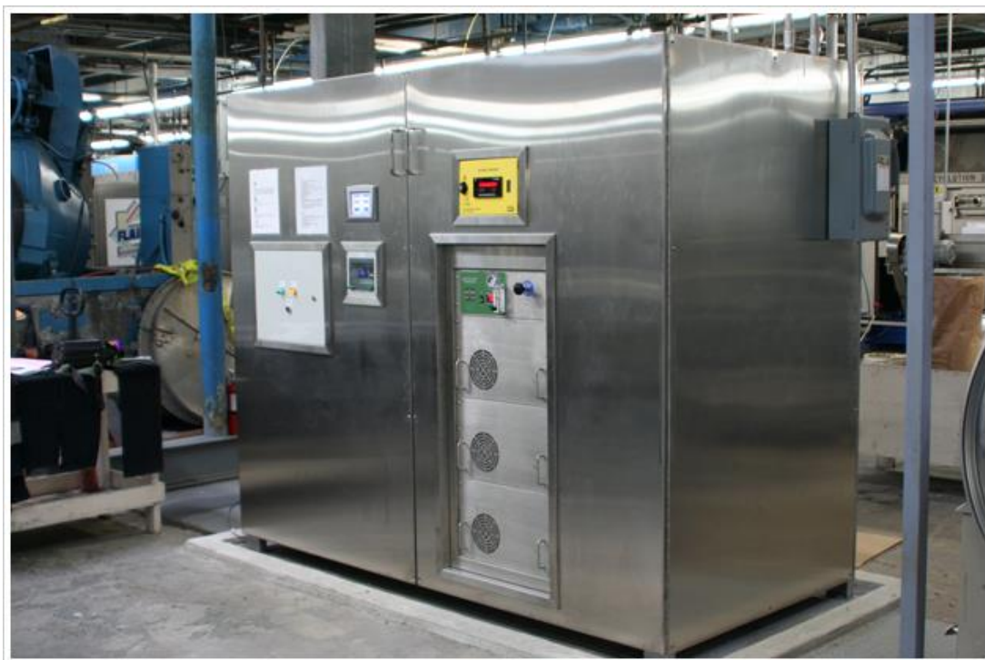
1.4.25-rasm. "OZONE DENIM" OLS-OC-1300– yuvish uskunasi
