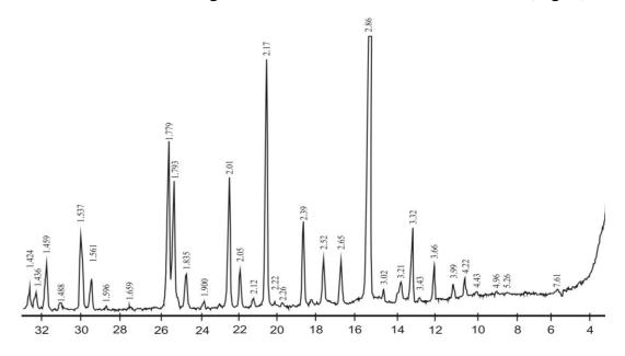
Figure 1. XRD pattern of dolomite "Shorsu"
