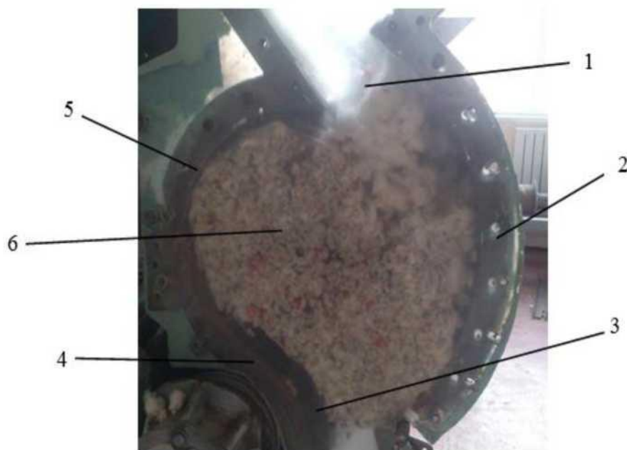
3.9- rasm. Arrali jin ishchi kamerasining o'zgartirilmagan ko'rinishi 1-chigitli paxta kirish yo'li, 2-old fartuk, 3-arrali silindr, 4-kolosnikli panjara, 5-orqa fartuk, 6-hom ashyo valigi.
