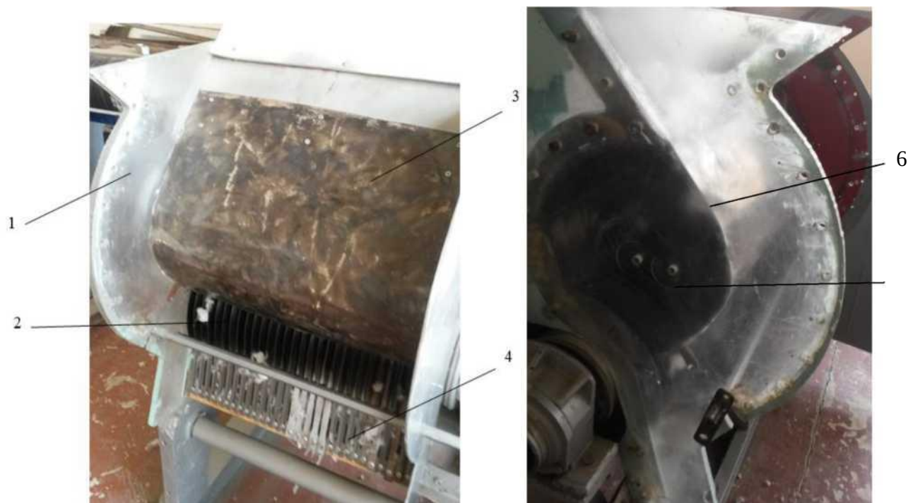
3.10- rasm. Yangi ishchi kameraga metal listni o'rnatilish jarayoni 1-yon devor o'rnida o'rnatilgan orgshisha, 2-arrali silindir, 3-metal list, 4-kolosnikli panjara, 5-ishchi kamera, 6-o'rnatilgan metal list.
