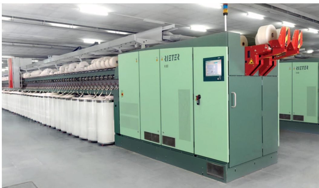
1.2-rasm. Rieter firmasining R 60 pnevmomexanik yigiruv mashinasi
