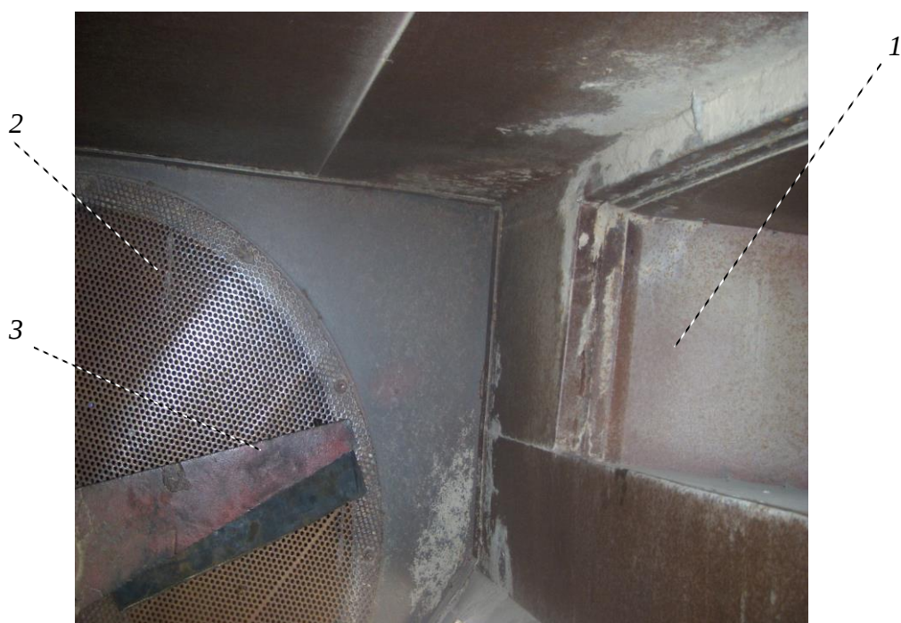
3.5-rasm. Yo'naltirgich o'rnatilmagan separator ishchi kamerasi 1-kirish quvuri; 2-to'rtli yuza; 3-sidirgich.
