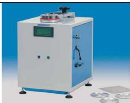
3.6-rasm. Air Tronic- matoni xavo o'tkazuvchanligini aniqlash asbobi
