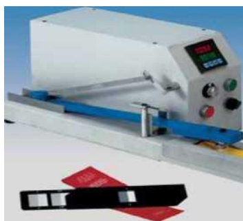
3.8-rasm. Crock-Meter- mato rangini ishqalanishga chidamliligini aniqlash asbobi
