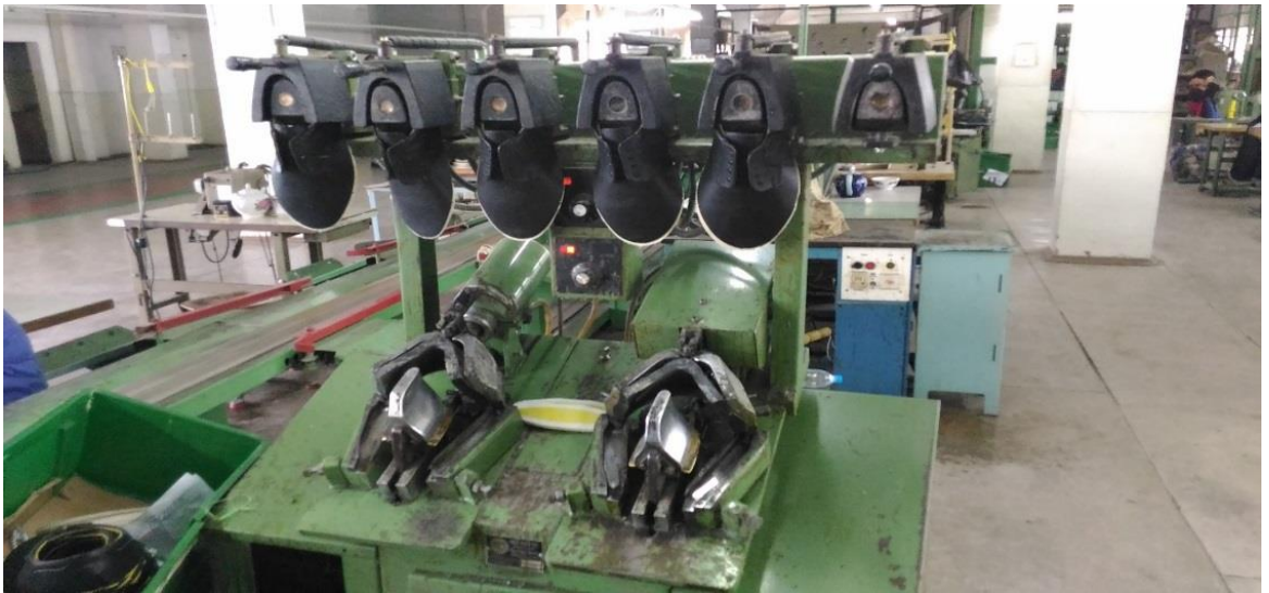
2.1.5-rasm. Tovon qismiga shakl berish mashinasi
