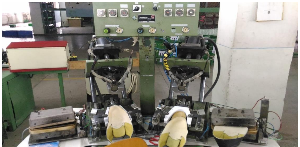
2.1.6-rasm. Burun qismiga shakl berish mashinasi
