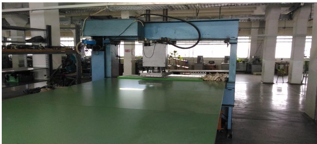
2.1.2-rasm. Press kesish mashinasi
