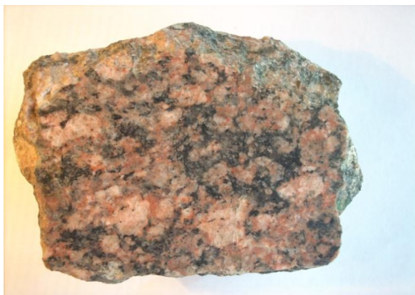
154-rasm. Yirik donali struktura (3-5mm)
