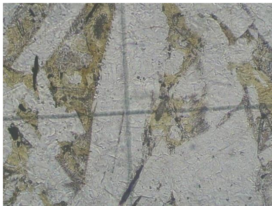
17-rasm. Biotit jigarrang, plagioklaz oq
