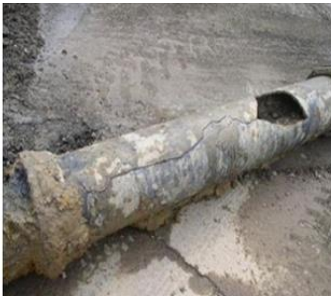
7-rasm. Gidravlik zarbalar natijasida cho'yan quvurning buzilishi
