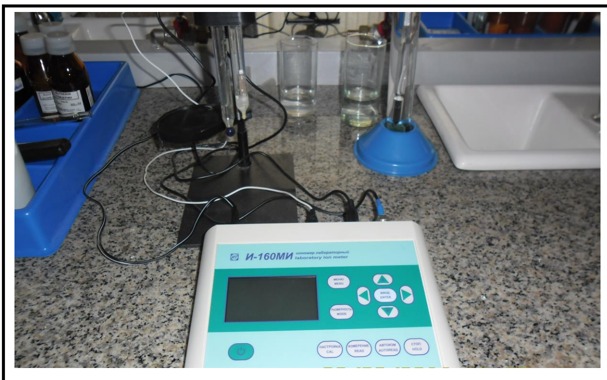
2-rasm. Mahuslot namunasidagi pH muxitini aniqlash uchun foydalaniladigan pH -My va TDL-100 termodatchik.
