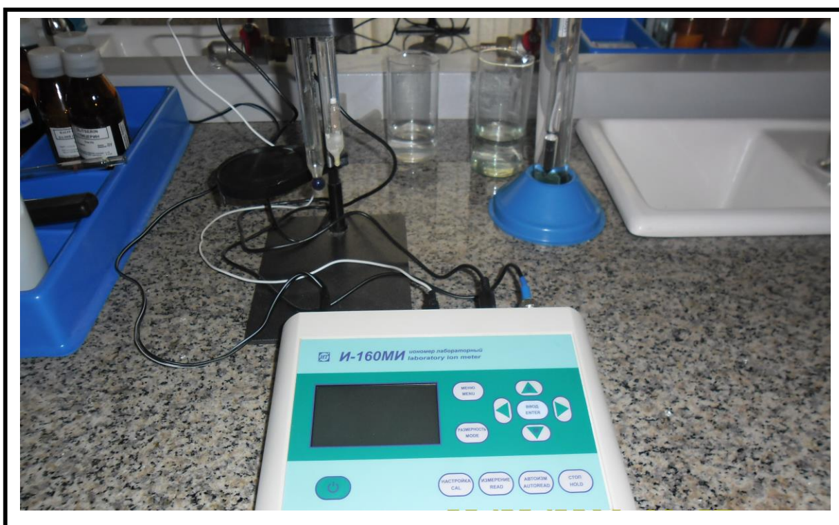
2-rasm. Mahuslot namunasidagi pH muxitini aniqlash uchun foydalaniladigan pH -My va TDL-100 termodatchik.
