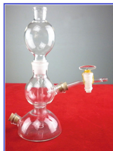
126-rasm. Kipp apparati
