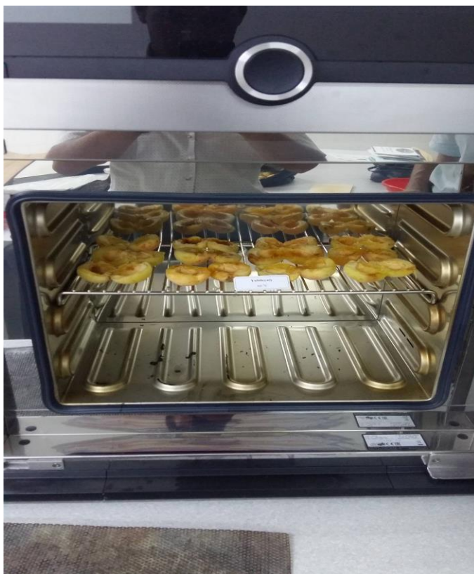
2.4.1-rasm. Laboratoriya sharoitida mahsulot namligini aniqlash.
