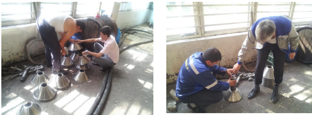
14-rasm. Seperatorni tarelkalarini tamirlash jarayon taxlili
