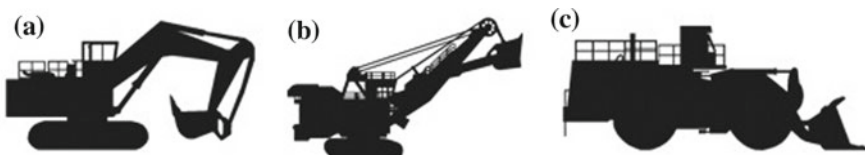
Fig. 1.2 Excavating equipment may include (a) hydraulic, (b) rope, and (c) front-end loaders (images from [17])
