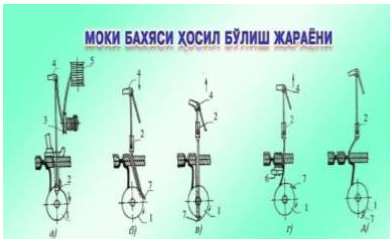
35-rasm. Moki baxya hosil qilish printsipti
