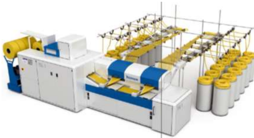
16 - rasm. “Trutzschler” firmasining TSL-1 piltabirlashtiruvchi mashinasi
