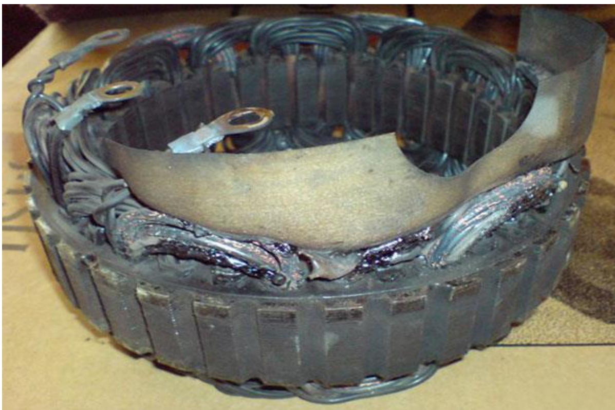
1.2-rasm.Stator cho'lg'aming shikastlanishi
