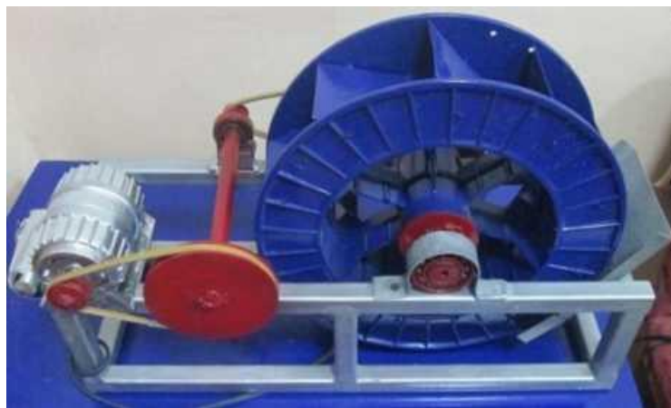
2-rasm. MikroGESning laboratoriya modeli
