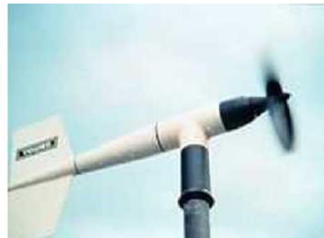
51-rasm. Uch (a) va to'rt(b)pallali hamdaparrakli(v) anemometrlar.
