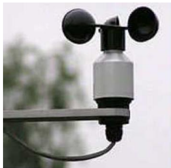
51-rasm. Uch (a) va to'rt(b)pallali hamdaparrakli(v) anemometrlar.
