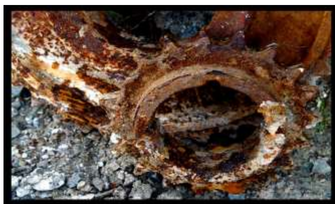
3-Rasm. Metallning tashqi muhit ta'sirida yemirilishi
