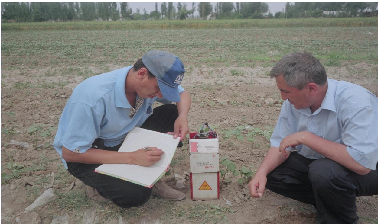
5-rasm. Tajribada namlikni VNP-1 nam o'lchagiya bilan o'lchash
