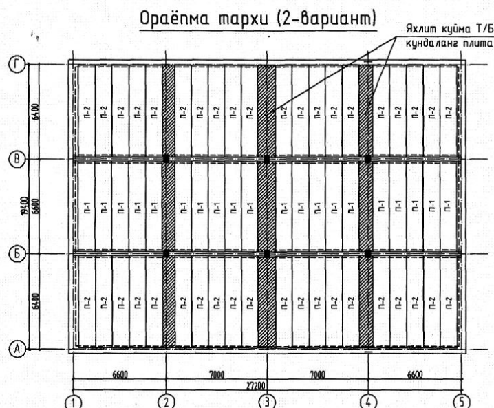
12.2-rasm 2. Ko`p qavatli temirbeton bino orayopmasining tarhi.
