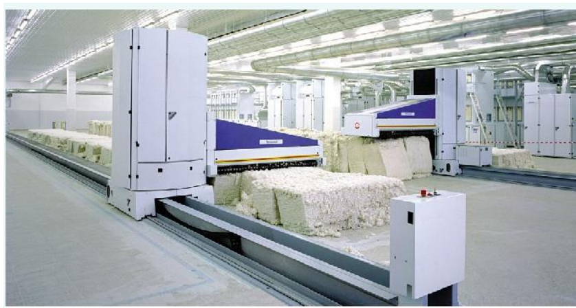
4-rasm. Tryuchler firmasining Blendomat BO-A universal toy titgich mashinasi
