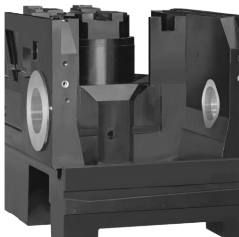
14.2-rasm. Mineralli quymadan tayyorlangan korpus detali.
