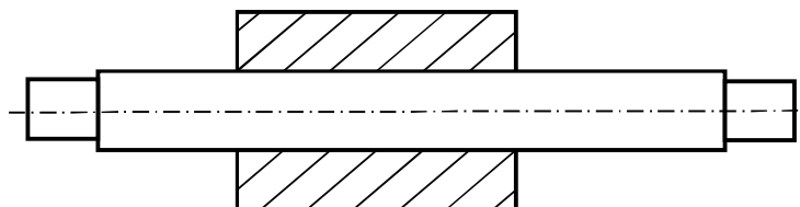
18.5-rasm. Konusli opravkaga o'rnatish.
