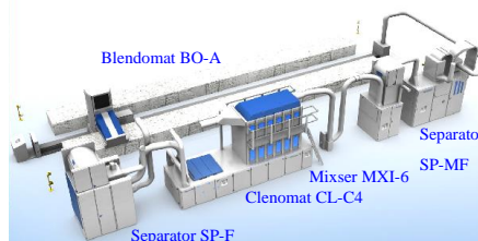
4.14-rasm. Tryuchler firmasining universal titish, tozalash, aralashtirish uskunalari tizimi
