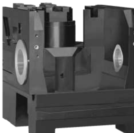
14.2-rasm. Mineralli quymadan tayyorlangan korpus detali.
