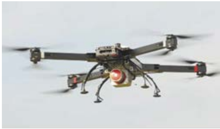
Fig.84. RiCOPTER unmanned system equipped with RIEGL air scanner
