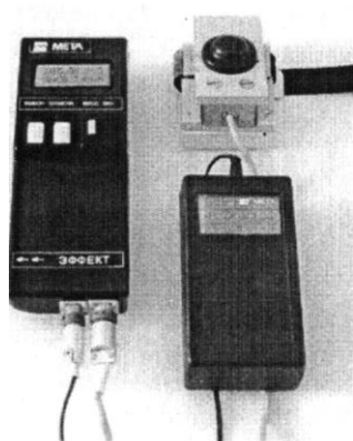
Tormoz tizimining samaradorligini aniqlovchi EFFEKT-02 jihozi
