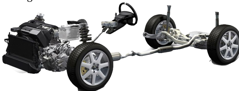
2.2-rasm. Yengil avtomobil yurish qismi.
